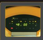
Low voltage 8Vdc digital control panel eliminating the risks of wet hands interfacing with mains.
