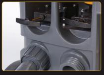
Twin gate vales for both solution and recovery tanks. Valves have been mounted horizontally to ensure no obstruction and debris filling the gate recesses which could cause leakage. Threaded ports allowing dump hose connection.
